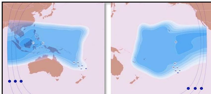
Figure 1: RAPIDCast- Current coverage on GE23 utilizing west and east Ku beams.
