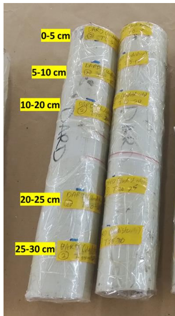
Figure 3 Preparation and leveling of core samples before cutting into 5 pieces (0-5, 5-10, 10-20, 20-25 and 25-30 cm)
